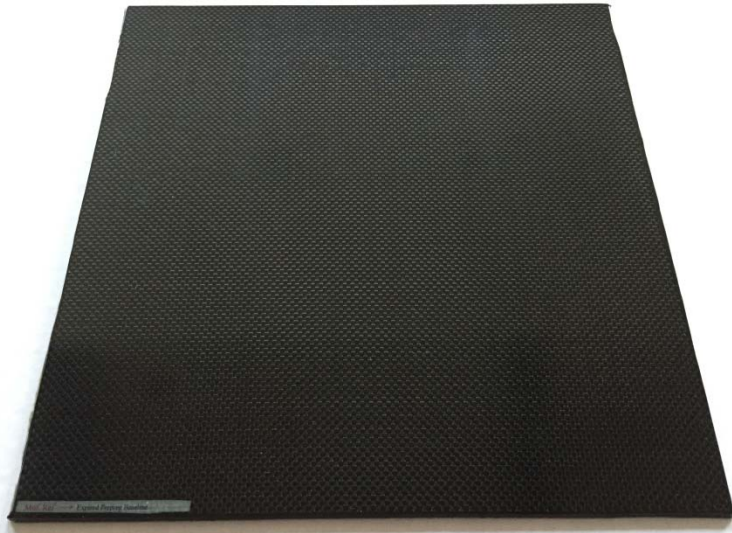
Panel made from fresh prepreg No void is visible on the panel surface
