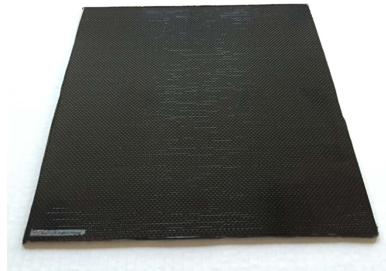
Panel made from expired (6-year old) prepreg High void content is visible on the panel surface (in addition, we had to use a very slow temp ramp up rate to cause the high void content)
